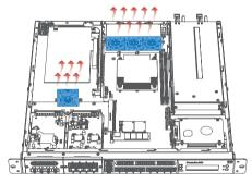
Users can define CPU fan and system fan speed and temperature profile in the BIOS menu. When the system is in idle or running less demanding tasks, smart fan is able to bring down the level of noise produced by rotating fans. The adjustable settings allow the PUZZLE-IN001 to be quieter during operation while extending the fan's lifespan, enhancing system stability and durability.
