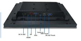
ALAD-171T-G is a new industrial touch display. ALAD-171T supports 17inches 1280\*1024 TFT LCD, with 5-wire resistive touch screen, optional projected capacitive touch. There are HDMI, DP, VGA video input, Audio input, optional support 2\*3W speakers.DC 9~36V wide power input. It is an industrial-standard multimedia display with a variety of installations that is fit for different applications.
