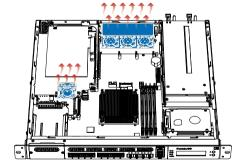
Users can define CPU fan and system fan speed and temperature profile in the BIOS menu. When the system is in idle or running less demanding tasks, smart fan is able to bring down the level of noise produced by rotating fans. The adjustable settings allow the Puzzle-A002 to be quieter during operation while extending the fan's lifespan, enhancing system stability and durability.
