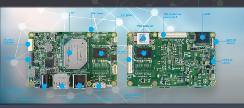
UP Core Plus is a credit card-sized board with high performance and low power consumption which features of the latest the Intel® Atom $^{\text{IM}}$  x5 / x $^{\text{7}}$  / Celeron / Pentium processor 64 bits up to 2.5 GHz.
